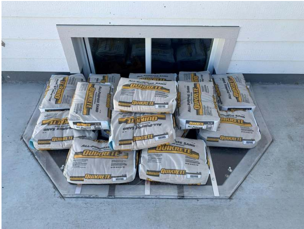
Photograph 3 - Specimen 1 Uniform Load Test
