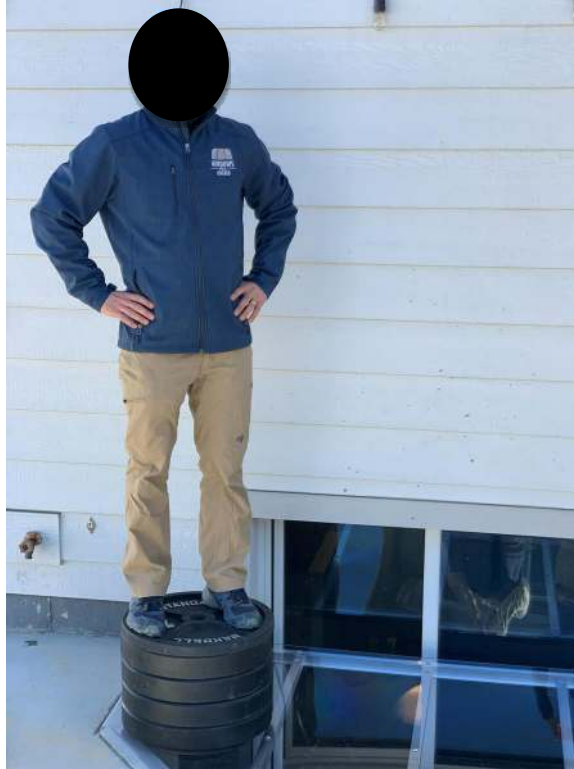
Photograph 8 - Specimen 1 Failure Point Load Test
