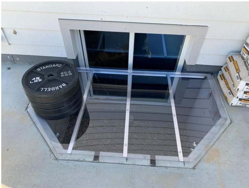
Photograph 6 - Specimen 2 Point Load Testing
