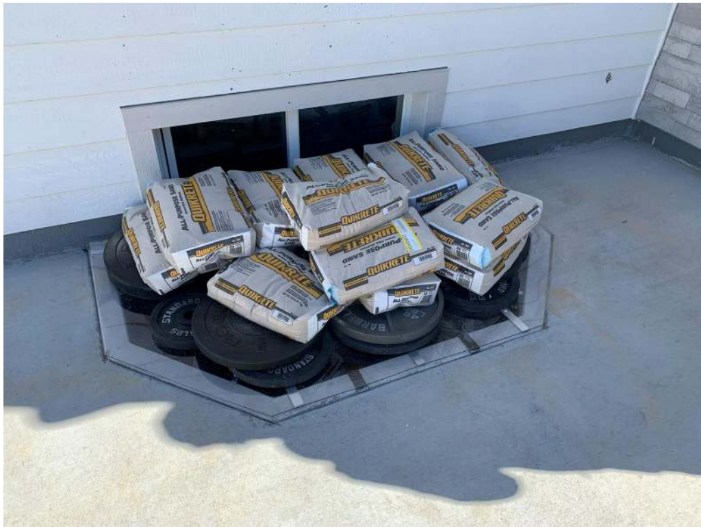
Photograph 7 - Specimen 1 Failure Uniform Load Test
