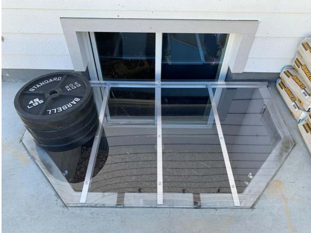
Photograph 4 - Specimen 1 Point Load Test
