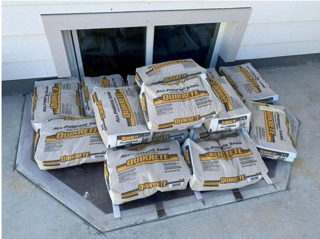
Photograph 5 - Specimen 2 Uniform Load Testing
